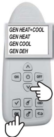
NOTE: after the INCLUSION procedure, wait 10 seconds before the next operation. Otherwise **WAIT** will appear on the display and every key will be inhibited.
