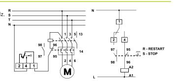
The circulation pump stops when the temperature drops below the detachment value.
