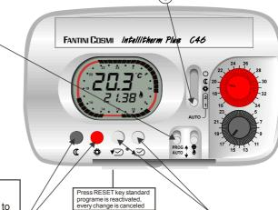
**5C** - Press the keys to colour the crown sectors. every time black key is pressed, the sector becomes black and the cursor moves on half an hour. every time the red key is pressed, the sector becomes red and the cursor moves on half an hour. to move the cursor along the crown without modifying the colour of the sectors, use the keys:
