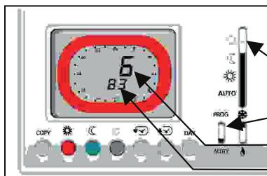
With Intellitherm C55 the user may verify how many hours the heating system has worked (relay closed - **ON**) the day before and since the last Intellitherm initialisation (i.e.: since last reset or battery fitting).
