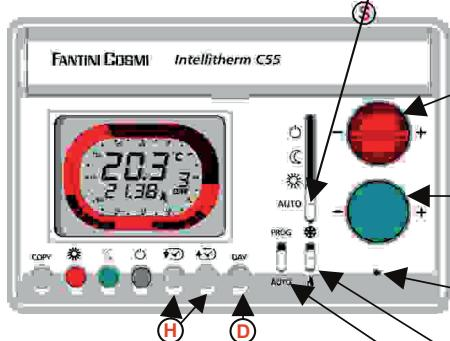
**2** Use the red keys to set the **COMFORT** temperature. The display will show the set temperature instead of the ambient temperature.
