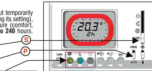
Once the time set has elapsed Intellitherm will resume the automatic program. To shorten or to cut out the "JOLLY" period before the set time, press a key of different colour than the one corresponding to display ring.
