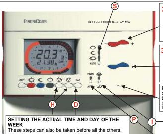
Using the red buttons, adjust the COMFOR t mode temperature. The display will show the temperature setting instead of the room temperature.
