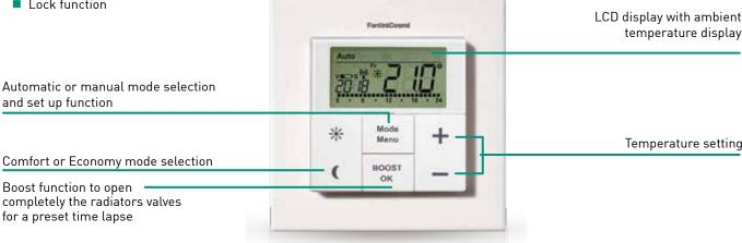
Thanks to the wireless technology C801 controls up to 8 radiators equipped with O81RF thermostats. C801 constantly sends inputs to the radiator thermostats based on the set values and the temperature readings in order to open or close the radiator valve.
