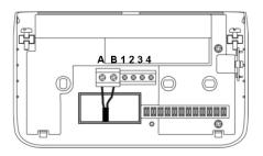
Connect the power wires coming from the actuator CH172D to terminals A and B, as shown in the figure. Flexible conductors with a max cross-section of 2.5 mm2 can fit in the terminals.
