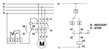
The circulation pump stops when the temperature drops below the detachment value.
