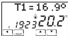
In the JOLLY program, the **TEMP** key alternates the display of the set temperature Tj and the hours left for the program to end: these two values can be changed using the ▲ and ▼ keys.
