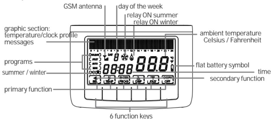
N.B.: the first time a key is pressed will have no effect other than turning the display light for it to be seen better.
