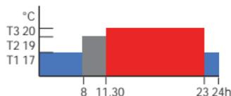
The value of the temperatures can be set using the **TEMP** function.
