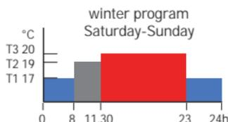
The value of the 4 temperatures can be set using the **TEMP** function.
