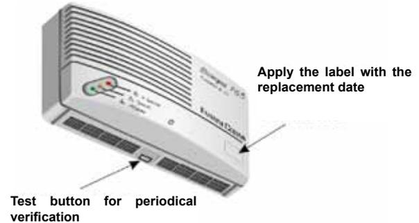
Sicurgas P63 is equipped with a test button for checking the system: button pressing activates a control procedure with 30 seconds duration. During this procedure the internal and external components of the system are checked.
