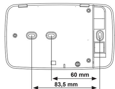
The Sicurgas P13 device, to be installed in bedrooms or rooms where the occupants spend most time, shall be placed quite near the occupants' breathing area, 0.8 to 1.2 m above the floor, at a point where the air flow will not be obstructed by pieces of furniture. Refer to the UNI 11522 installation standard.
