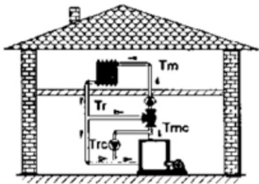
**3-WAY ROTOR POWER-OPERATED MIXING VALVE**
