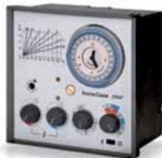
detected by special probes provided for the purpose. Temperature values are sent to the control unit which according to the set programming determines the delivery water temperature value to be sent to the system to keep the set ambient temperature constant.
