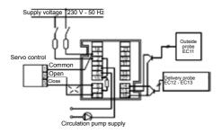
2 - Wiring diagram for motor-operated mixing valves with servo controls powered with voltages other than 230V 50 Hz
