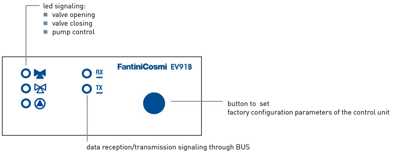
EV91B is an electronic device that regulates the mixing valve opening and closing based on the desired temperature and the read temperature. The device works properly only when it's connected through a two-wire serial bus (FANBUS) to a Master device called EV90 or EV87.
