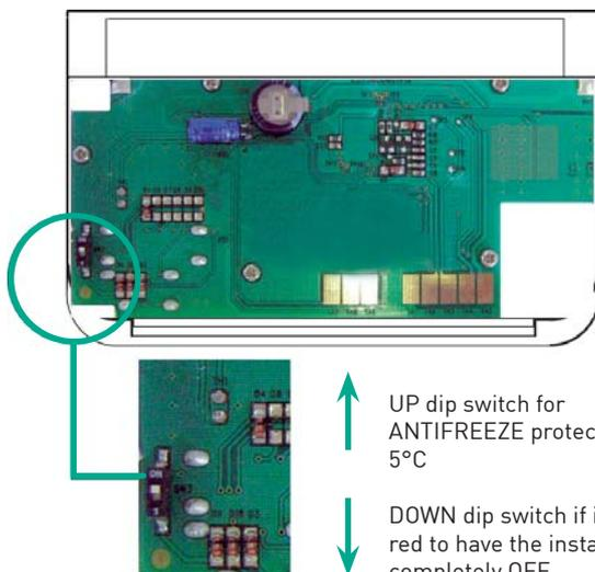
UP dip switch for ANTIFREEZE protection - 5°C
