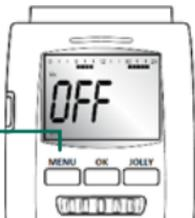
When the valve is closed, the anti-calcification function still remains active. To deactivate the function, go to AUTO mode.
