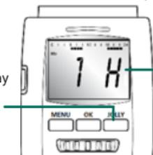
During operation in JOLLY mode, the wheel selector and **OK/JOLLY** keys are inactive. To annul JOLLY mode, press the **MENU** key.
