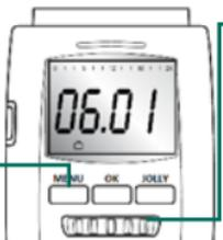
The set temperature or the chosen valve status (OFF-closed, ON-open) will appear on the display, together with the holiday symbol
