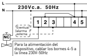
**RELE A IMPULSOS PASAJE DE CORRIENTE PARA EL MANDO DE UNA VALVULA A REARME MANUAL NORMALMENTE ABIERTA NA (PUENTE ARRIBA)**
