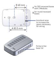
After fixing and connecting the appliance (see paragraph 4), refit the lid on the base, making sure that the two teeth on the lid perfectly fit in the two upper guides. Retighten the fixing screw and apply the sticker in the seat indicating the date of replacement.
