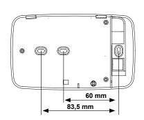
The Sicurgas P13 device, to be installed in bedrooms or rooms where the occupants spend most time, shall be placed quite near the occupants' breathing area, 0.8 to 1.2 m above the floor, at a point where the air flow will not be obstructed by pieces of furniture. Refer to the UNI 11522 installation standard.
