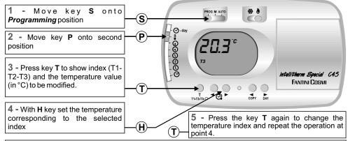
PROGRAMMING OF OPERATING TIME, COMBINED WITH TEMPERATURE INDEXES
