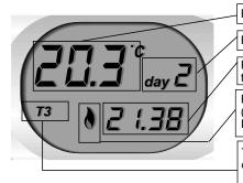
Read of ambient temperature (functions as a thermometer)
