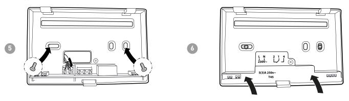
Tighten the screw shown and hook the body onto the panel on the wall.
