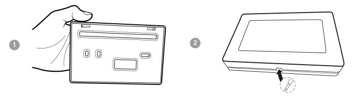
Remove the insulating protection by unscrewing the specific waterproof screw.
