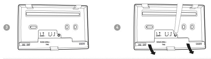
Make the electrical connections (refer to the "Electrical connections" paragraph) and secure the panel to the wall with the supplied screws.
