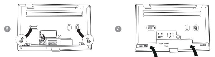
Tighten the screw shown and hook the body onto the panel on the wall.
