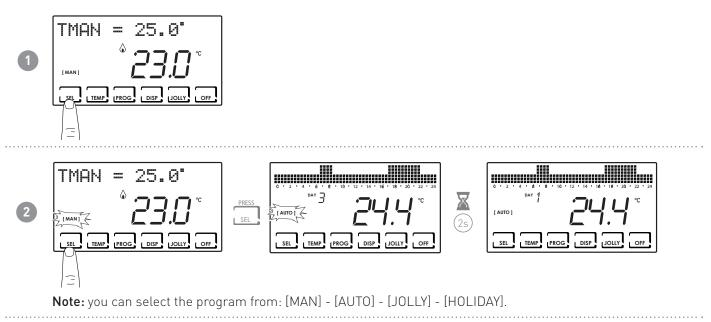
Pressing the DISP key allows you to display certain parameters set according to the active operating program.
