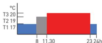
The value of the temperatures can be programmed using the TEMP function. The temperature profile (hourly variation) can be programmed using the PROG function.
