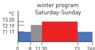
The value of the 4 temperatures can be programmed using the TEMP function. The temperature profile (hourly variation) can be programmed using the PROG function.
