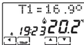
Pressing TEMP in the JOLLY program allows you to modify its temperature using the keys ▲ and ▼. Press ◀ to go back to the page displaying the hours, allowing you to modify them using ▲ and ▼.
