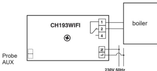
N.B. When CH193WIFI is disconnected, the boiler contact remains in its current position. Unscrew the lid to connect the auxiliary probe.
