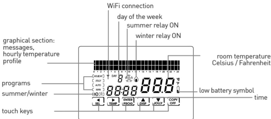
N.B.: to switch on the display, press in the middle; if no other keys are pressed, the display switches off after 2 seconds; if other keys are pressed, the display will switch off after remaining idle when the time set in the parameter LIGHT ON expires (see Chap. 6 CONFIG. PG03).
