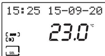
When the keyboard is locked, you can only press the SEL key. Pressing SEL allows you to enter the set password and unlock the keyboard.
