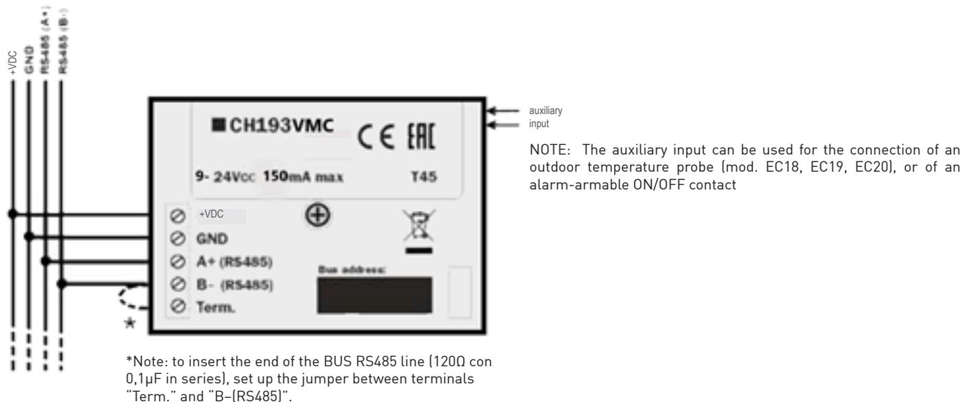
All of the VMC machines code AP200xx feed remote control CH193VMC
