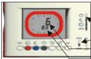
With Intellitherm C75 the user may verify how many hours the heating system has worked (relay closed - **ON**) the day before and since the last Intellitherm initialisation (i.e.: since last reset or battery fitting).
