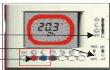
Once the time set has elapsed Intellitherm will resume the automatic program. To shorten or to cut out the "JOLLY" period before the set time, press a key of different colour than the one corresponding to display ring
