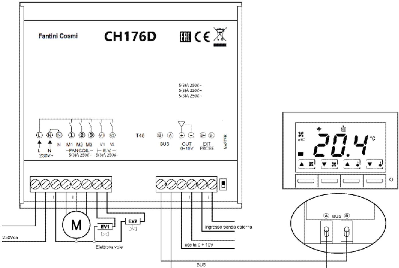
ESEMPIO DI COLLEGAMENTO TRA CH133AR2+CH176D A PIÙ FAN-COIL (DA 2 A 5)
