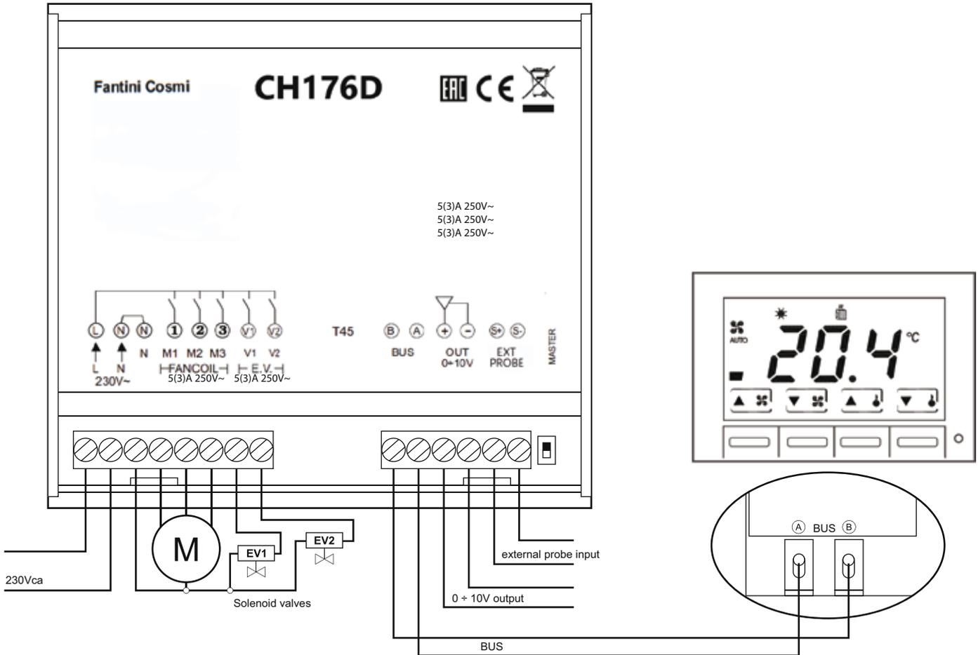
CONNECTION EXAMPLE BETWEEN CH133AR2+CH176D AND FEW FAN-COILS (FROM 2 TO 5)
