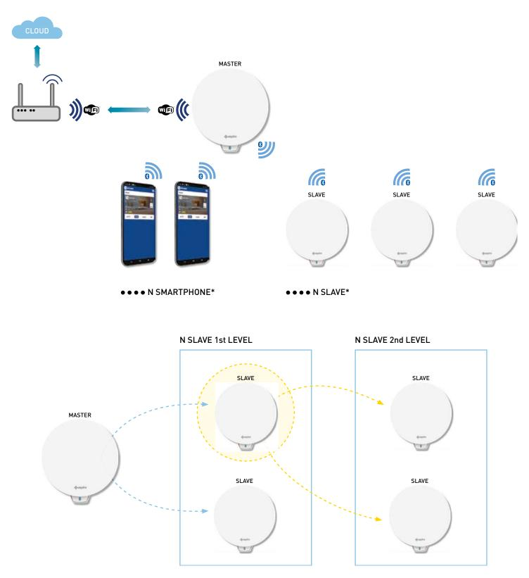
The Ecocomfort 2.0 Smart system may consist of a Master and several Slave units communicating with each other via Bluetooth Low Energy.
