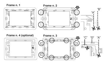
cut 4, 8 or 12 tabs according to type of cover plate
