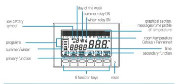
N.B.: pressing a key once has no effect aside from switching on the light on the display to have a hetter view
