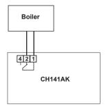
PLEASE NOTE: when CH141AK is disconnected, the boiler contact remains in its current position.
