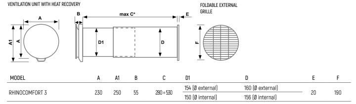
For wall thicknesses between 250 mm and 280 mm, cut the pipe and use a standard external grille (not included)
