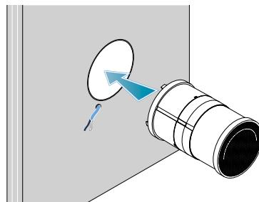
**BEFESTIGUNG DER ELEKTRONIKEINHEIT und STROMANSCHLUSS**
